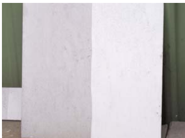
The right of the board was coated COAT PT301, the left was not coated.
